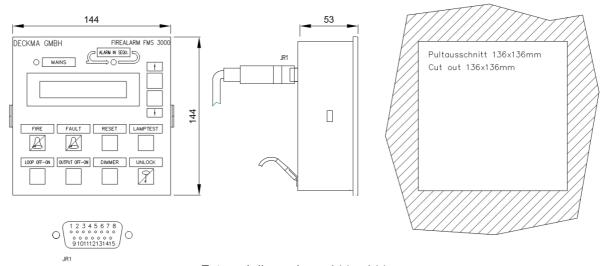
External dimensions: 144 x 144mm installation depth 53mm plus the corresponding D-SUB connector.
